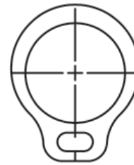
Lug Design For Sizes SH-12 thru SH-23
