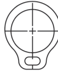
Lug Design For Sizes SH-12 thru SH-23
