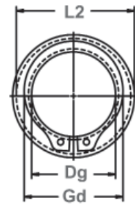
Clearance Diameter & Gaging Diameter Released in Groove.
